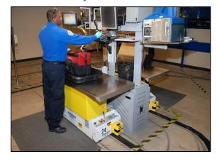
Figure 3-3. Vanderlande FLEET Autonomous Checked Baggage Management System at DFW
