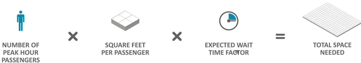
Figure 2-2: Key Calculation Used for Space Planning at Airports with Time LoS Considered
