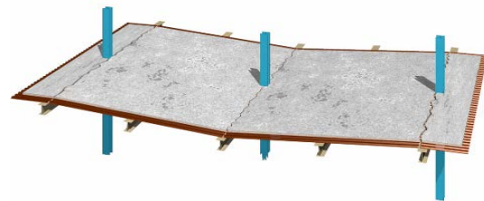
Figure B-13. Catenary Cable Floor Support System
