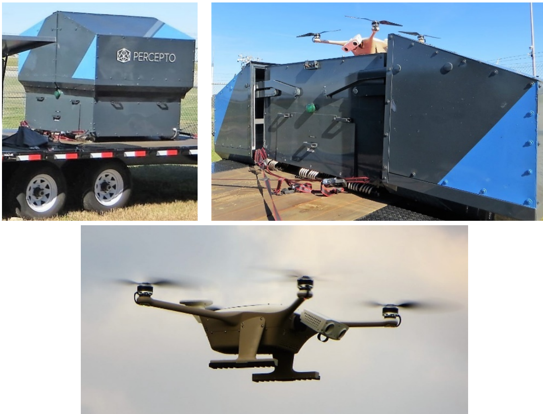
Figure A-3. Percepto System Components (clockwise from top left): Base Station (Closed), Base Station (Open), Sparrow in Flight
