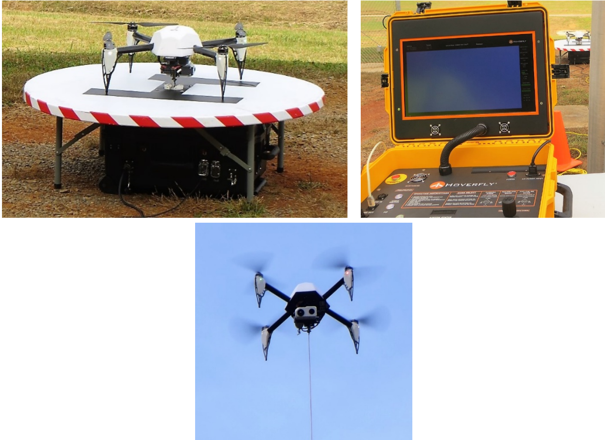
Figure A-6. HoverFly System Components (clockwise from top left): LiveSky on Its Base, Field Launch Kit, LiveSky in Flight
