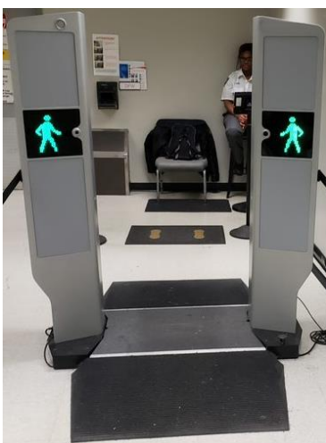
Figure 3-6. Walk-Through MMW Detection Technology
