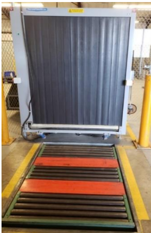
Figure 5-4. An X-ray Machine Designed to Scan Bulky Items
