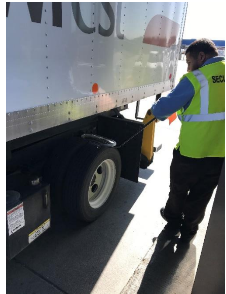
Figure 4-2. Example of an Undercarriage Mirror in Use
