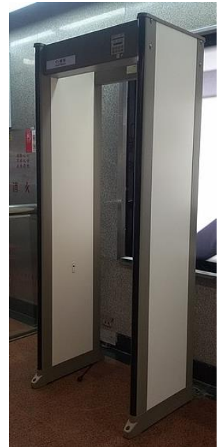
Figure 3-5. Example of a Walk-Through Metal Detector
