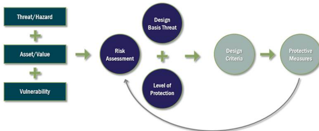
Figure 6. Iterative Protective Design Process
