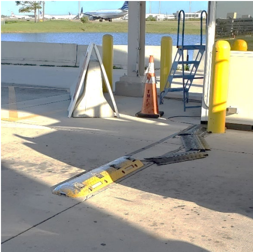
Figure F-6. Portable UVIS Installation
