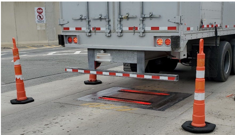
Figure D-6. UVIS Scanning a Vehicle Undercarriage
