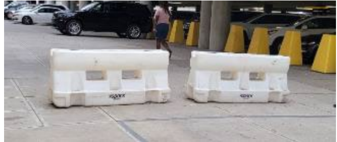
Figure 8-12. Example of Water-Filled Plastic Barriers
