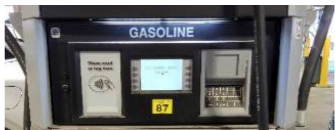
Figure 6-4. Example of a Fuel Pump with Access Control
