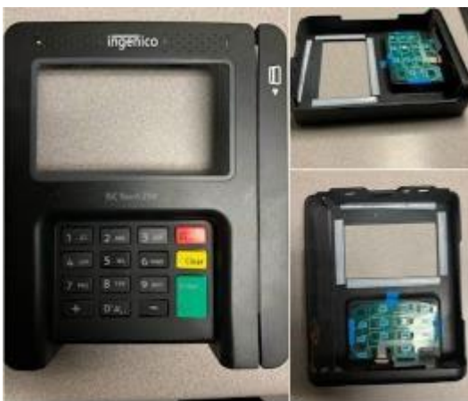
Figure 6-7. Example of a Card Skimmer
