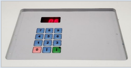
Figure 4-29. SAN Filing System Control Panel
